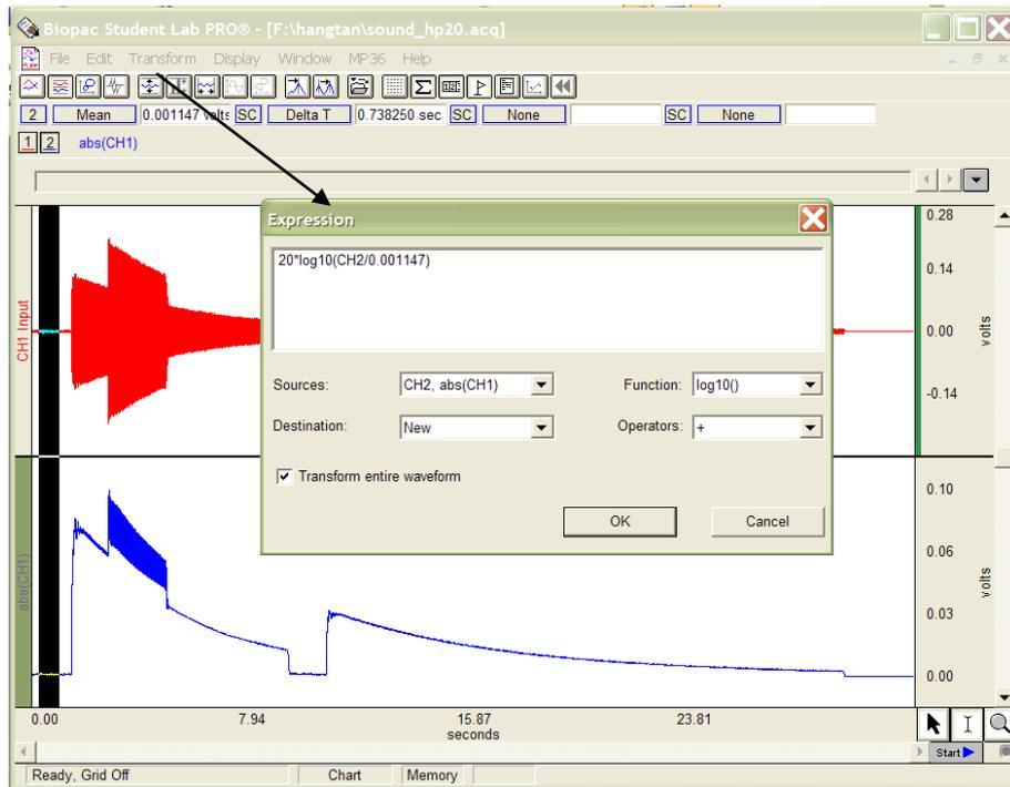
Figure 11. Determining the background pressure and calculating the sound level.
