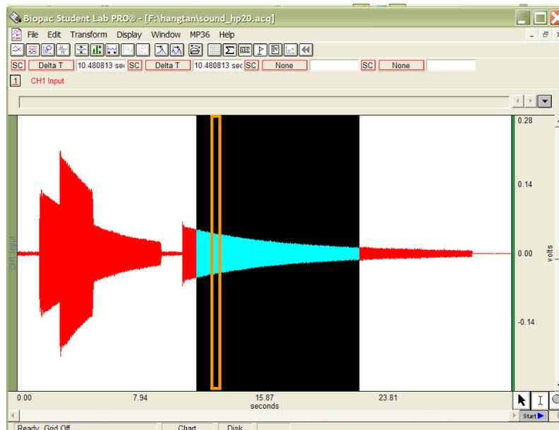
Figure 9. Selecting an interval for the spectrum calculation.
