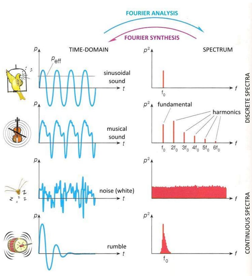
Figure 3. Time-domain waveforms and spectra of different sounds.
