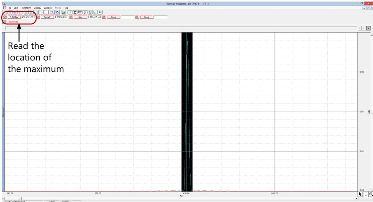
Figure 8. Determining the location of the spectral peak.
